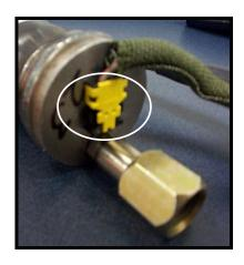
If access to either of these connectors is not possible due to deformation of the seat assembly or the fuselage, it is acceptable to cut the cable that connects to the inflator assembly.
